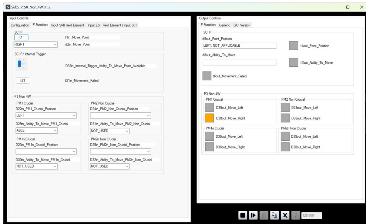
Please note: The simulator does not 'simulate' the physical driving of the point machine. In physical terms, it is expected that when driving from 'left' to 'right', the PM1 Crucial will detect the following sequence LEFT > NO\_END\_POSITION > RIGHT. These changes of the input value D22in\_PM1\_Crucial\_Position have to be done manually by the tester.
